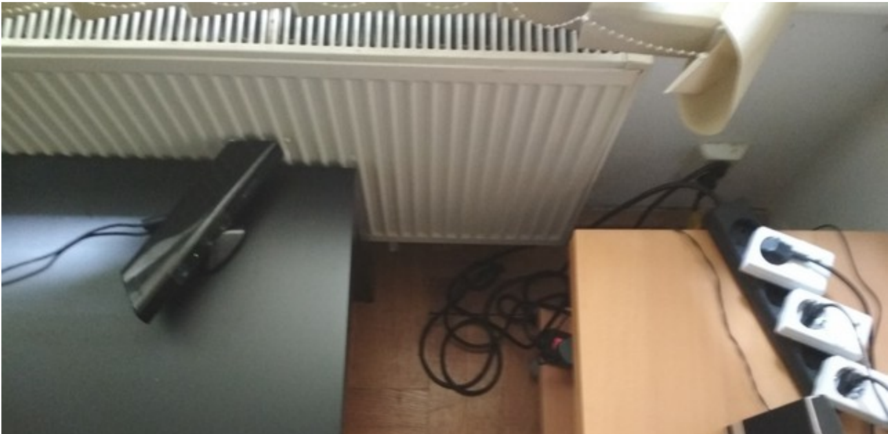
Fig. A.6 – Final positioning of Kinect camera at an angle to the wall (~2 meters)
