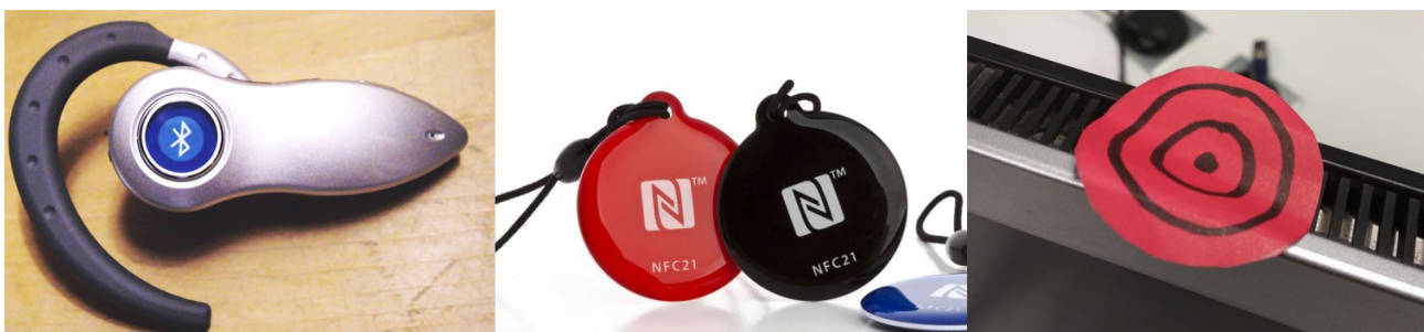
Fig. 14 – Objects with activation symbols (like logos) for Bluetooth (left) and NFC (middle) which indicate a standardized technology. The target right was used in HomeNodes with the NFC tag underneath and not using the trademarked logo. The tags themselves do not have the trademark.
