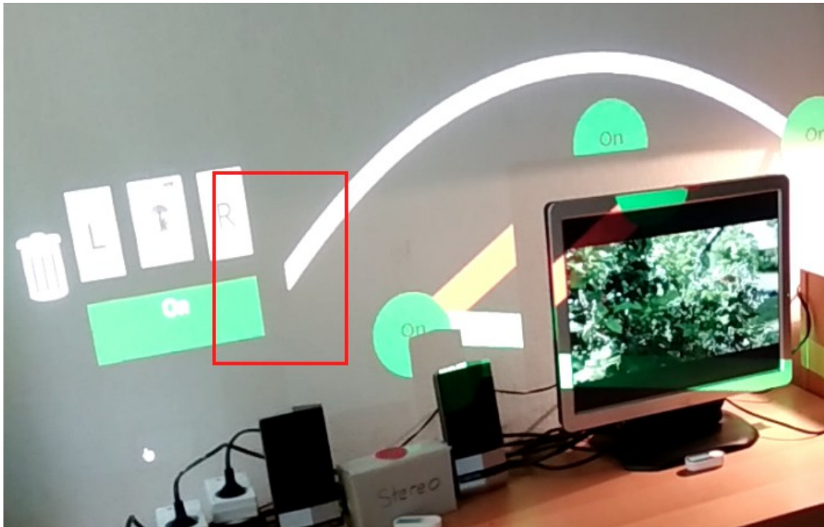
Fig. 9 – Red box indicates the point where the UbiDisplays surfaces meet. The coordinates of the visual elements in the HTML and CSS are off-screen and used to align both surfaces.
