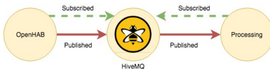
Fig. 10 – MQTT communication channels in HomeNodes
